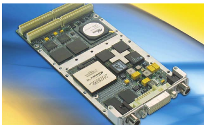
Aitech's new PMC drives dual 2- or 3-D-video displays from independent data streams at resolutions as high as 1536×2048 pixels.
